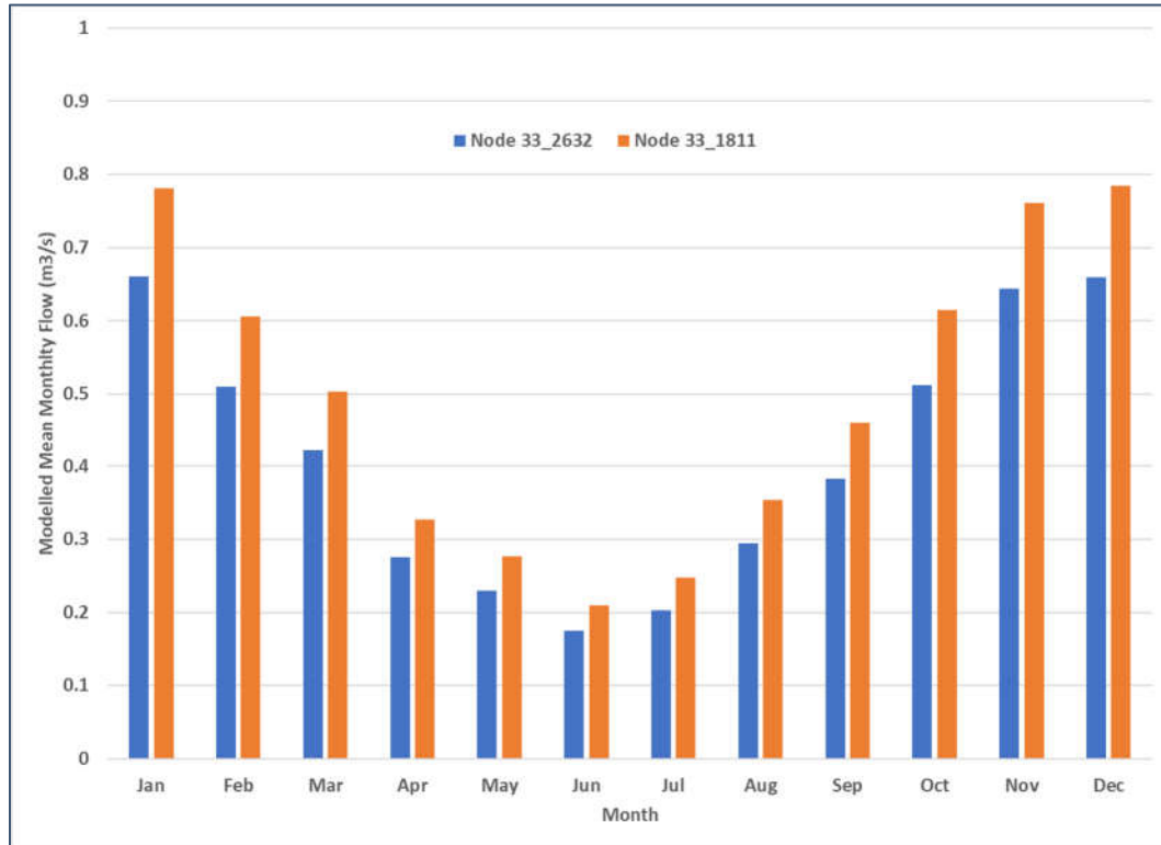
Figure 9-8 Model-Estimated Mean Monthly Flows in the Two Streams That Drain the Proposed Development Area
